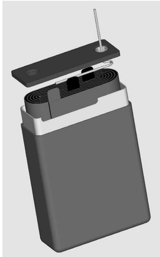
Fig. 2. A cross-section view of the coiled electrode configuration (A). An assembly view of a typical battery with the cover and electrode coil partially removed showing the attachments in the headspace (B).
